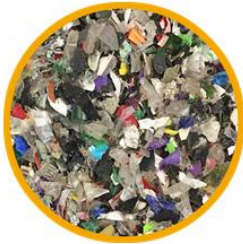
Plastic waste is “pre-conditioned” through a shredding and dry-cleaning process.
