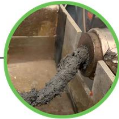
Plastic waste is “hybridised” through a heat extrusion process.
